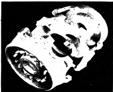
FIG. 11-2.—Aluminum Company of America forged aluminum-alloy crankcase for a Pratt and Whitney 14-cylinder radial engine.
