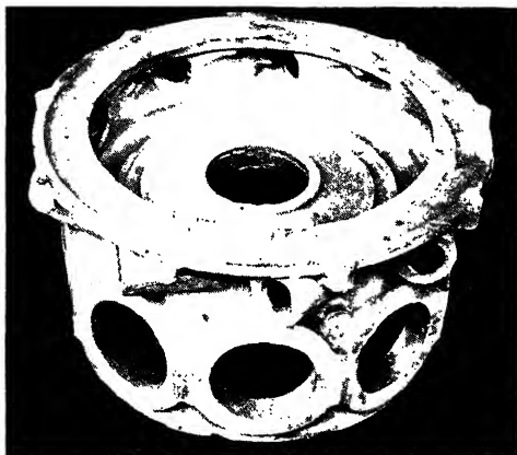
FIG. 11-1.—American Magnesium Corporation, magnesium alloy, AM7-4HT, crankcase for a Lycoming nine-cylinder radial engine.
